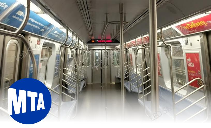
Starting in 2018, the New York City Transit department began to install LED Smart, custom LED lighting system to retrofit their Alstom, Bombardier and Kawasaki R142, R142A, and R160 cars. MTA NYCT is in the process of retrofitting these 3,138 cars with the best in LED technology, the LED Smart RLR Series.
